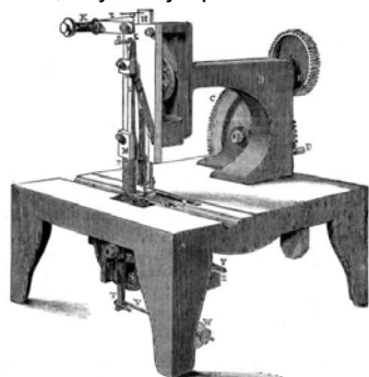
THE SINGER MACHINE, AUGUST 12, 1851. Earliest model filed in Patent Office. Reproduced from the SCIENTIFIC AMERICAN of November 1, 1851.
